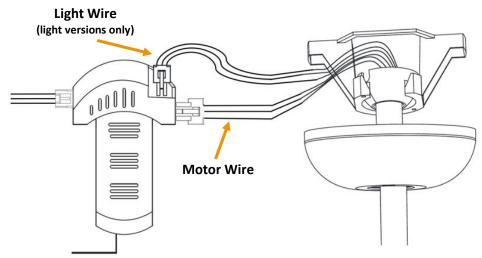
17. Align the canopy with the screw holes on the mounting bracket and twist to secure in place. **NOTE:** You may need to loosen/tighten the screws to secure correctly.
