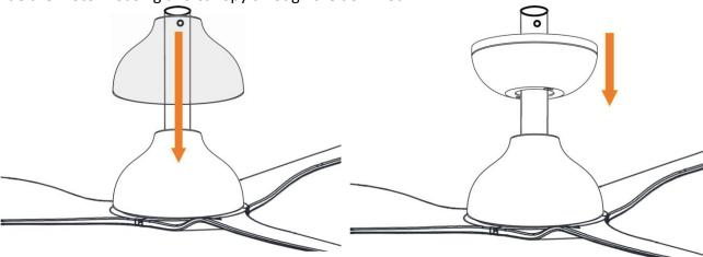
14. Place the hanging ball on top of the down rod and secure it with the ball pin and screw.
