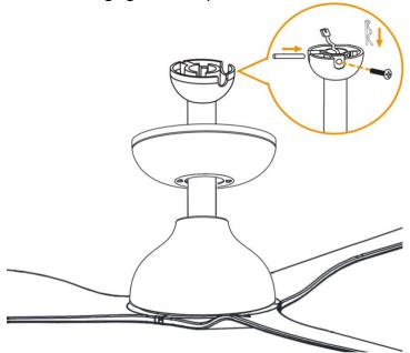
15. Hang the fan into hanging bracket. Align ball groove on hanging ball with ridge on hanging bracket. Ensure hanging ball sitting into hanging bracket correctly. If fan doesn't sit properly, hold the downrod and twist it until fan has been secured into hanging bracket.
