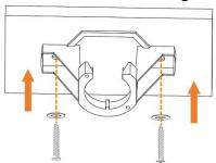
2. Attach the blades to the motor by aligning the screw hole and affix the blade to the motor with a blade screw.
