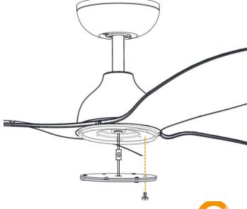
g. Align the grooves of the Light Ring with the grooves of the Light Kit Plate and twist into place.
