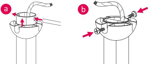
7. Hang the fan into hanging bracket. Align ball groove on hanging ball with ridge on hanging bracket. Ensure hanging ball sitting into hanging bracket correctly. If fan doesn't sit properly, hold the downrod and twist it until fan has been secured into hanging bracket.
