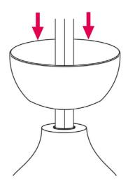
6. Place the hanging ball on top of the down rod and secure it with the ball pin and two screws. **CAUTION**: Secure one screw through holes on the hanging ball and the down rod.
