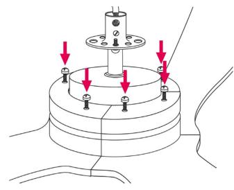
4. Take off side screws from downrod holder. Put the motor housing and plate washer on downrod holder and secure it with 6 screws.
