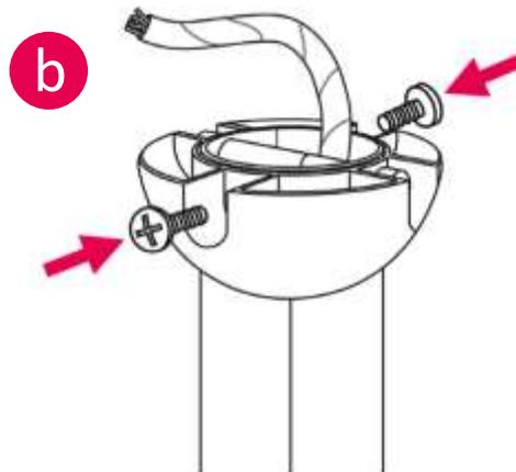
14. Hang the fan into hanging bracket. Align ball groove on hanging ball with ridge on hanging bracket. Ensure hanging ball sitting into hanging bracket correctly. If fan doesn't sit properly, hold the downrod and twist it until fan has been secured into hanging bracket.
