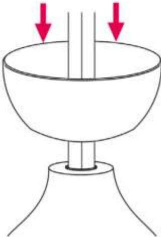
13. Place the hanging ball on top of the down rod and secure it with the ball pin and two screws.
