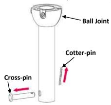
3. Feed the main motor and light wire (light version only) plug up through the inside of the down rod, then insert the down rod into the downrod holder. Gently push the cross-pin through the holes aligned with the base of the downrod holder and downrod. Insert cotter pin into cross pin and secure downrod with two set screws.
