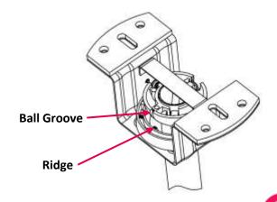
9. Place receiver in the hanging bracket and follow the wire diagram to connect wires and connectors. Connect power, receiver and the fan as per electrical wiring diagram.
