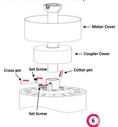
4. Snuggle the coupling cover down onto the top of the motor housing. **CAUTION: DO NOT** remove rubber gasket on top of the coupling cover.
