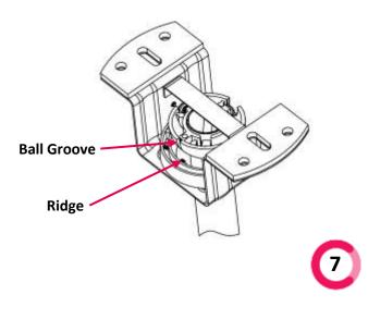
Place receiver in the hanging bracket and follow the wire diagram to connect wires and connectors. Connect power, receiver and the fan as per electrical wiring diagram.
