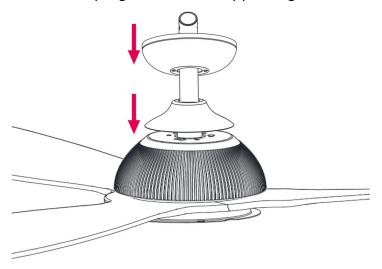
15. Place the hanging ball on top of the down rod and secure it with the ball pin and screw.
