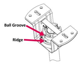
17. Place receiver in the hanging bracket and follow the wire diagram to connect wires and connectors. Connect power, receiver and the fan as per electrical wiring diagram.
