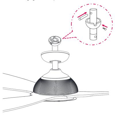
16. Hang the fan into hanging bracket. Align ball groove on hanging ball with ridge on hanging bracket. Ensure hanging ball sitting into hanging bracket correctly. If fan doesn't sit properly, hold the downrod and twist it until fan has been secured into hanging bracket.
