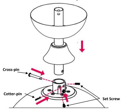
5. Snuggle the coupling cover down onto the top of the motor housing. Put the canopy through the downrod.
