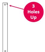
4. Feed the main motor and light wire (light version only) plug up through the inside of the down rod, then insert the down rod into the downrod holder. Gently push the cross-pin through the holes aligned with the base of the downrod holder and downrod. Insert cotter pin into cross pin and secure downrod with two set screws.
