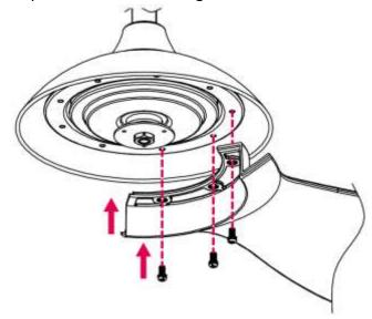
10. Hang the fan into hanging bracket. Align ball groove on hanging ball with ridge on hanging bracket. Ensure hanging ball sitting into hanging bracket correctly. If fan doesn't sit properly, hold the downrod and twist it until fan has been secured into hanging bracket.
