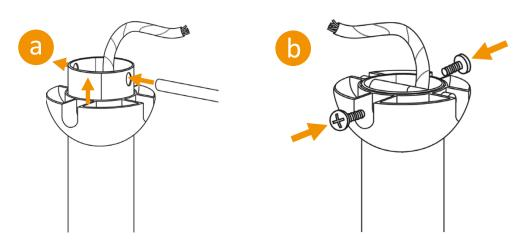
14. Hang the fan into hanging bracket. Align ball groove on hanging ball with ridge on hanging bracket. Ensure hanging ball sitting into hanging bracket correctly. If fan doesn't sit properly, hold the downrod and twist it until fan has been secured into hanging bracket.
