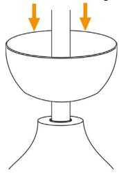
13. Place the hanging ball on top of the down rod and secure it with the ball pin and two screws. **CAUTION**: Secure one screw through holes on the hanging ball and the down rod.
