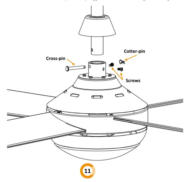
11. Snuggle the coupling cover down onto the top of the motor housing. **CAUTION**: **DO NOT** remove rubber gasket on top of the coupling cover.
