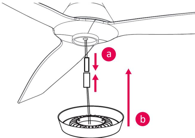
13. Hang the fan into hanging bracket. Align ball groove on hanging ball with ridge on hanging bracket. Ensure hanging ball sitting into hanging bracket correctly. If fan doesn't sit properly, hold the downrod and twist it until fan has been secured into hanging bracket.
