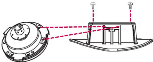
7. Remove side screws from extension rod. Put the motor housing through the extension down rod and secure with screws.
