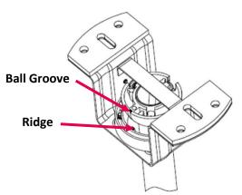
9. Place the receiver in the hanging bracket and follow the wiring diagram to connect wires and connectors.
