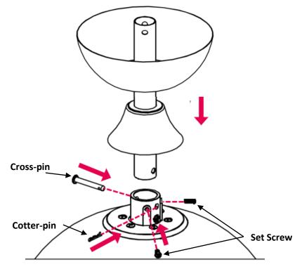
4. Snuggle the coupling cover down onto the top of the motor housing. Put the canopy through the downrod.
