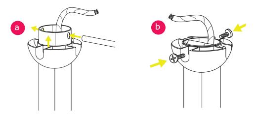
8. Face slot on hanging ball to the middle of the hanging bracket. Place hanging ball into the bracket.
