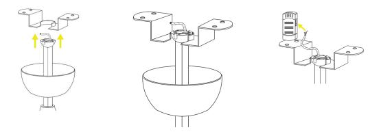
9. Place the receiver on top of the hanger ball and connect the wires.
