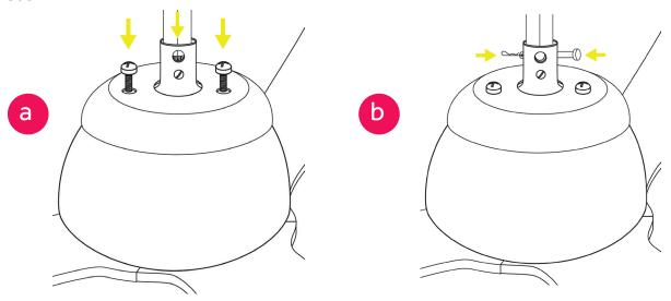
5. Snuggle the coupling cover down onto the top of the motor housing. CAUTION: DO NOT remove rubber gasket on top of the coupling cover.
