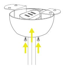
12. For the light model - hold the diffuser to the bottom of the motor and rotate clockwise until it locks into place.
