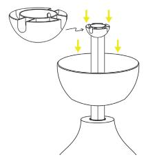
7. Place the hanging ball on top of the down rod and secure it with the ball pin and two screws. CAUTION: secure one screw through holes on the hanging ball and the downrod.
