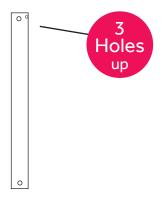
Feed the main motor wire plug up through the inside of the downrod, then insert the downrod into the motor bush. Gently push the cross-pin through the holes aligned with the base of the motor bush and downrod. CAUTION: DO NOT force the cross-pin, gently wiggle and rotate it until it glides through both holes. Replace the cotter-pin on the other side of the cross-pin to secure the downrod to the motor bush. Tighten up both cross screws to make the downrod rigid in the motor bush.
