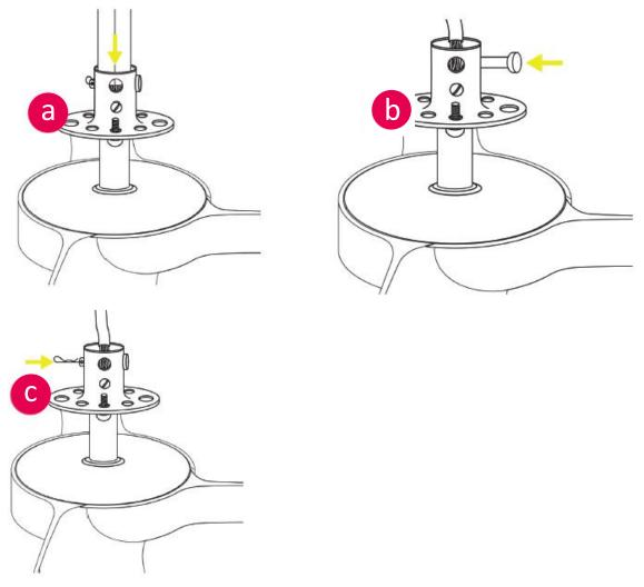
9. Snuggle the coupling cover down onto the top of the motor housing. **CAUTION**: **DO NOT** remove rubber gasket on top of the coupling cover.
