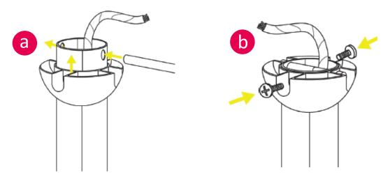
12. Face slot on hanging ball to the middle of the hanging bracket. Place hanging ball into the bracket. Rotate down rod and ensure the slot on hanging ball aligns with the ridge on the hanging bracket.
