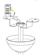
14. Connect power, receiver and the fan as per the electrical wiring diagram.
