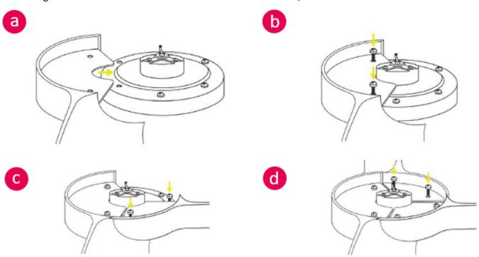
**48" MINI ONLY:** Align the blades with screw holes on the top of the motor, and secure with screws.
