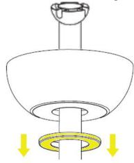
16. Place the canopy over the bracket, align the canopy holes with the screws and tighten. Clip it in to secure it onto the canopy.
