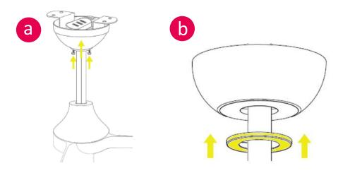
17. Hold the diffuser to the bottom of the motor and rotate clockwise until it locks into space.
