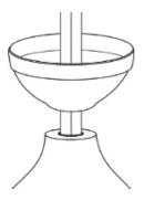
11. Place the hanging ball on top of the down rod and secure it with the ball pin and two screws. **CAUTION**: Secure one screw through holes on the hanging ball and the down rod.
