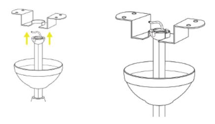
13. Place the receiver on top of the hanger ball and connect the wires.
