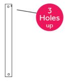
7. Feed the main motor and light wire plug up through the inside of the down rod, then insert the down rod into the motor bush. Gently push the cross-pin through the holes aligned with the base of the motor bush and down rod.
